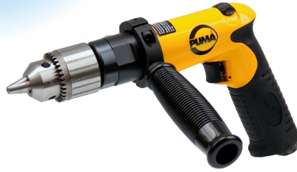
AT-4341R 700 rpm 1/2" reversible air drill-0.6hp
