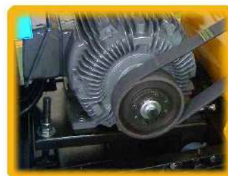
槓桿式皮帶調整結構 Easy maintenance mechanism
